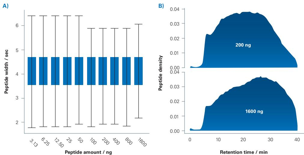
**A)** Narrow average peak widths for 3.13 ng to 1600 ng K562 tryptic digest. Boxes and whiskers correspond to 50% and 1.5 times the interquartile data range, respectively (Outliers not shown).
