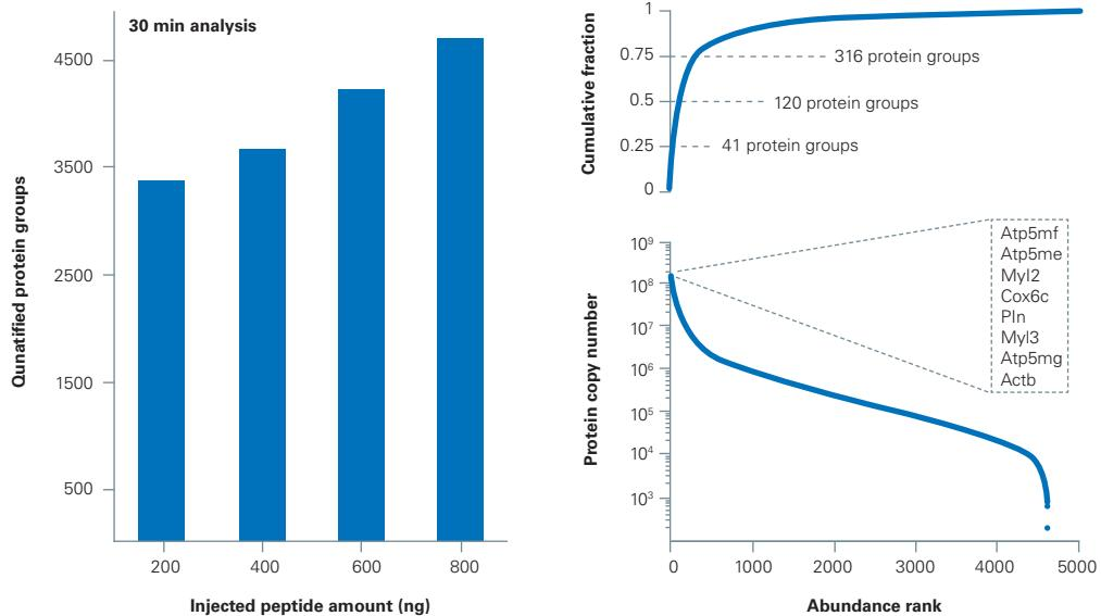
Rapid cardiac tissue proteomics. The new timsTOF HT featuring the well-known dia-PASEF technique enables robust and accurate quantitation of proteomes in tissues at only 30 min LC-MS gradient time. Different amounts of a murine heart proteome digest were analyzed in triplicates with short liquid chromatography gradients and dia-PASEF.
