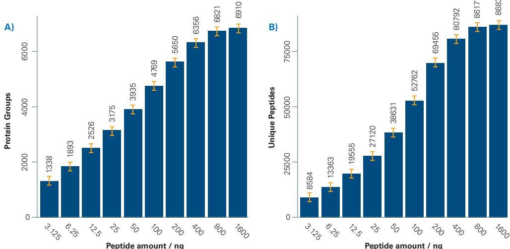
**A)** The TIMS XR allows for increased ion capacity for sample loads beyond 200 ng. Reproducible identification of ~ 6900 protein group identifications and more than 86,000 unique peptide identifications
