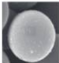
ARION® particle 1.3 µm
