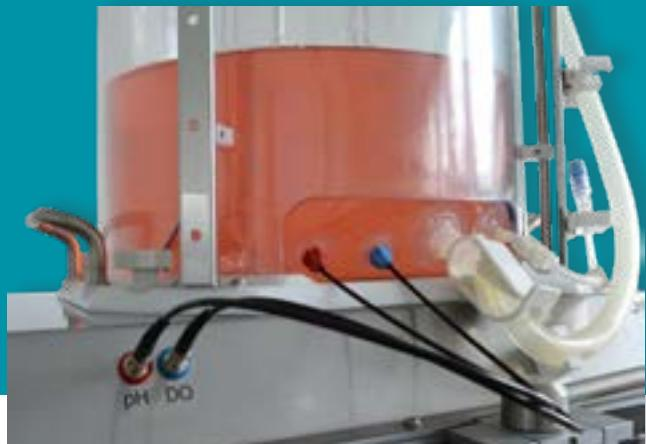
The SB10-X is an orbital shaken benchtop bioreactor system for the cultivation of human, animal, insect and plant cells in a single-use bag. It consists of six modules (excluding the bag) and has a working volume from 4 litres up to 12 litres. The SB10-X can be used in research, process development or as a pilot scale bioreactor.
