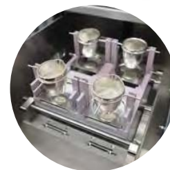
Equal temperature distribution on all 4 samples
