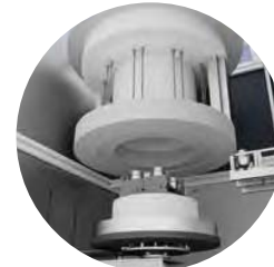
closed oven with lift bottom for precise temperature control
