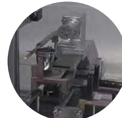
Autosampler handles samples automatically
